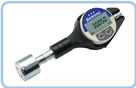
SmartPlug with ceramic contacts
